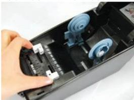
Transmissive sensor (Gap, Media sensor)
